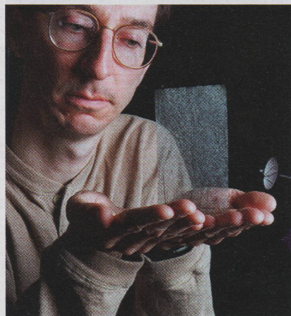
A NASA researcher holds a rigid, lightweight carbon-fiber material suitable for building a large and efficient solar sail. Without such materials, the sails would be impossible.
